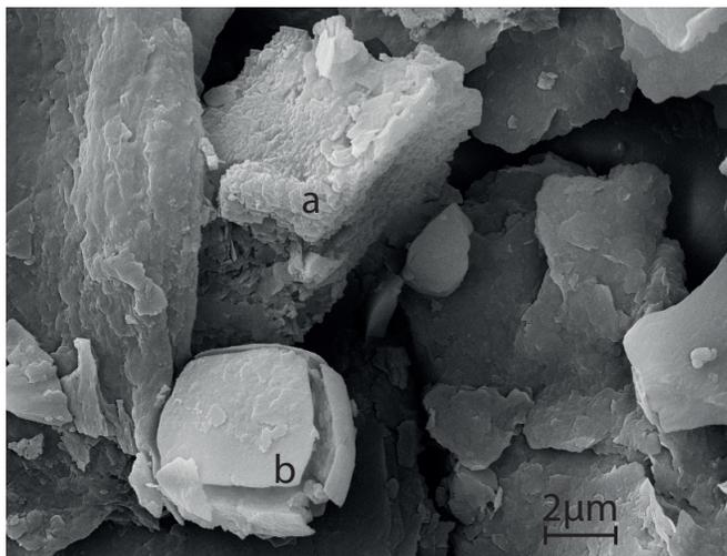
**Fig. 4.** SEM photos of bulk sediment from 137 cm depth in core Co1260 showing endogenic calcite (**a**,  $\text{CaCO}_3$ ) and pyrite (**b**,  $\text{FeS}_2$ ). The broken structure of the pyrite is probably due to sample pre-treatment and heating to  $50^\circ\text{C}$ .
