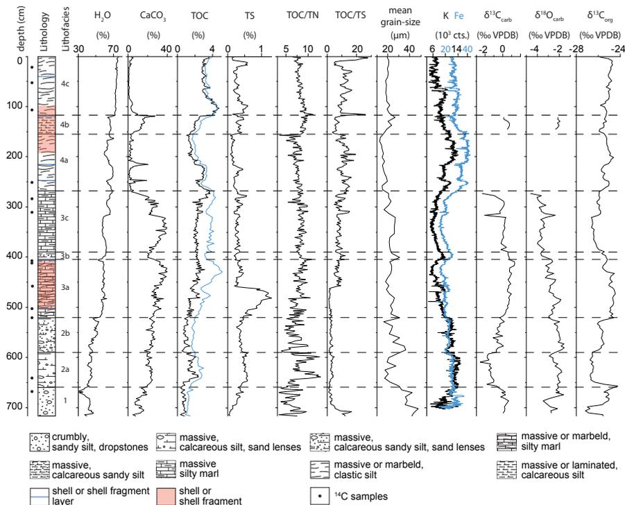
**Fig. 3.** Positions of <sup>14</sup>C samples, lithology, lithofacies, water content, calcite (CaCO<sub>3</sub>), TOC (black line) and CaCO<sub>3</sub> adjusted TOC (blue line), TS, TOC/N, TOC/TS, mean grain-size, Potassium (K) and Iron (Fe) counts, δ<sup>13</sup>C<sub>carb</sub>, δ<sup>18</sup>O<sub>carb</sub>, and δ<sup>13</sup>C<sub>org</sub> of core Co1260.
