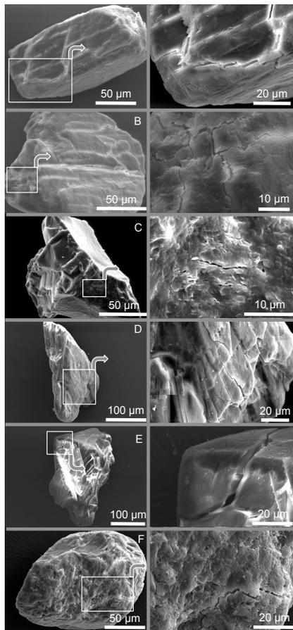
**Fig. 3.** SEM imagery with zoomed features of quartz grains (63–125  $\mu\text{m}$  fraction) from topmost 12 m of lake sediments.
